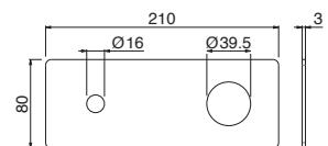
Cover plate for 2 hole basin mixer OTEN range, mod. V30050.
