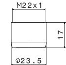
Aerator M22x1 for bidet mixer TIMEA range (**only** for mod. V16070), SLATE range (**only** for mod. V14070), PARANÀ range (**only** for mod. V22070), INDO (mod. V24070) and OTEN (**only** for mod. V30070 e V30071).
